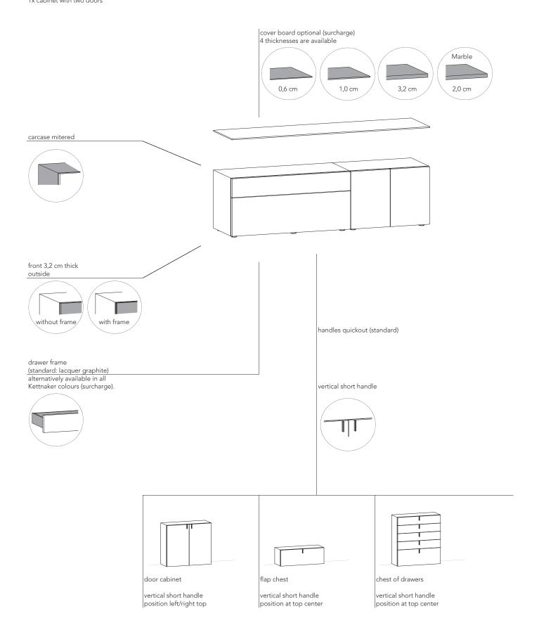
possible with 2-door cabinets without middle cheek. pair of doors width 80 cm can be divided in 30/50 cm (40/40 cm standard)
